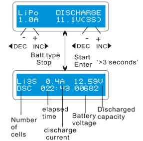
**\*Voltage balancing and monitoring during the discharge**
