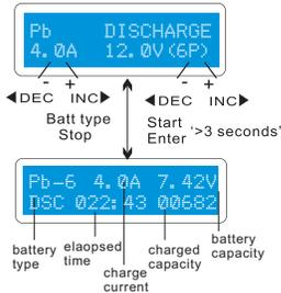
Set discharge current on the left and final voltage on the right.The discharge current ranges from 0.1 to 5.0A.
