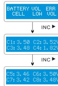
The peocessor found that the voltage of one of the cell in the Lithium battery pack is too low.
