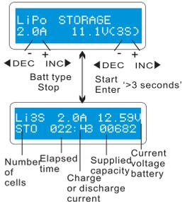
You can set up the current and the voltage of the battery pack to be charged.The current will be used for charge or discharge the battery to reach the 'storage' level of voltage.
