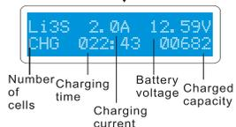
The screen shows the present situation during charge process.To stop charging press Batt type key once.
