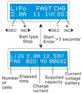
You can set up the charging current and the voltage of the battery pack being charged.As you press **Start/Enter** button the voltage confirmation will be displayed.And then,If you confirm the voltage and current,press **Start/Enter** button again to **start/Enter** button again to start charging.
