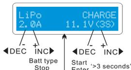
The left side of the first line shows the type of battery you select at the users setting.The value on the left side of second line sets a charge current and the value on the right side of second line sets the voltage of the battery pack. After setting the current and voltage press Start key for more than 3 seconds to start the process.(Charge current:0.1~10.0A,Voltage:1~6series)
