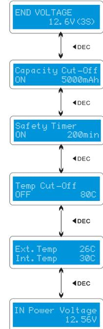
The internal temperature of the charger and the temperature of battery being charged.
