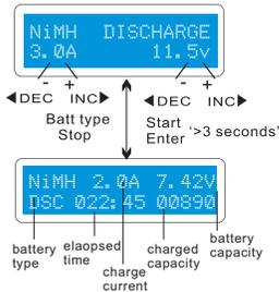
Set discharge current on the left and final voltage on the right.The discharge current ranges from 0.1 to 5.0A and the final voltage ranges from 0.1 to 25.0V.To start the process,press **Start/Enter** key for more than 3 seconds.
