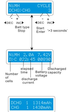
To stop the process,press **Batt.Type/Stop** key once. You can change the discharge or charge current by pressing **Start/Enter** key once during the process.The audible sound indicates you the end of process.
